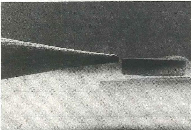
Magnetic levitation achieved by high temperature transition superconductors.
