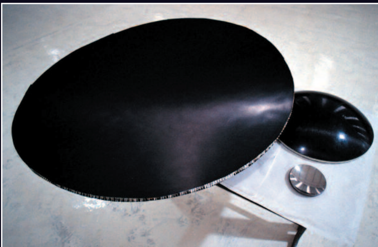
Carbon-fiber factory prototype of the mirrors.
