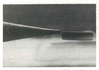
Magnetic levitation achieved by high temperature transition superconductors. (Photo from the Instituto de Materiales, UNAM)
